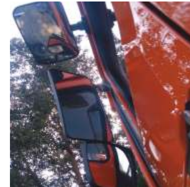
Side close proximity mirror Normal rear view mirror Wide angle rear view mirror
